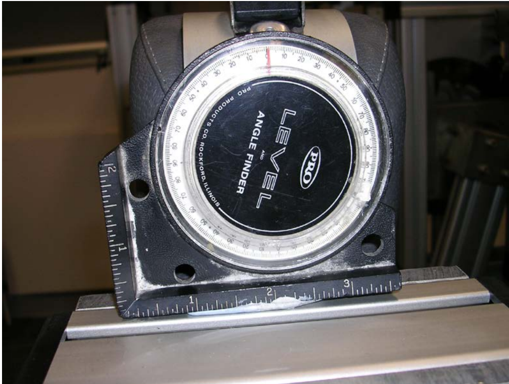
Figure 3: goniometer attached to the lever arm used for the JPS tests.
