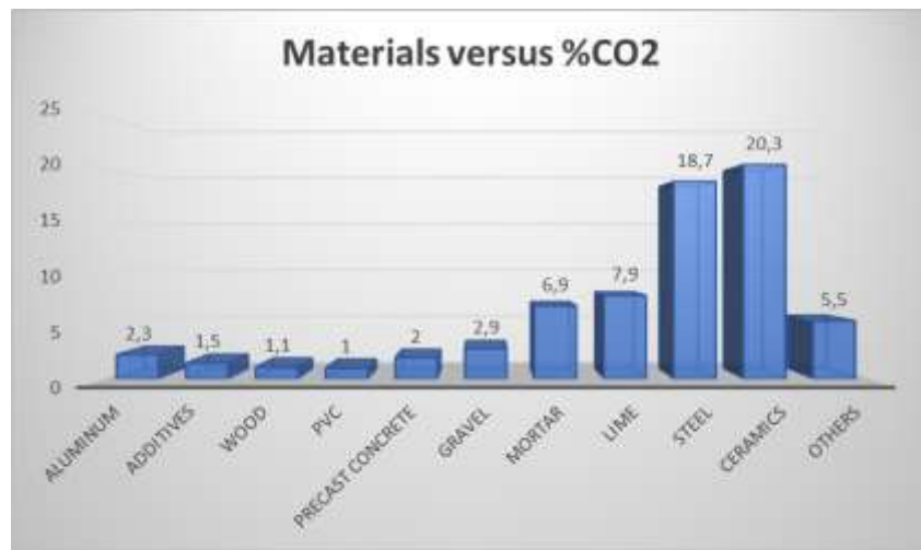
Figure 1. Contribution of the materials required for the construction of 1m on the CO 2 emissions associated with its manufacture.
