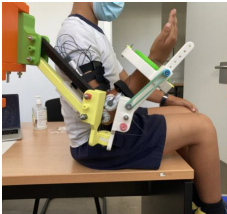
Figure 6 Exoskeleton and sEMG configuration. Exoskeleton and surface electromyography (sEMG) sensors arrangement for elbow flexion assistance (assistive mode).
