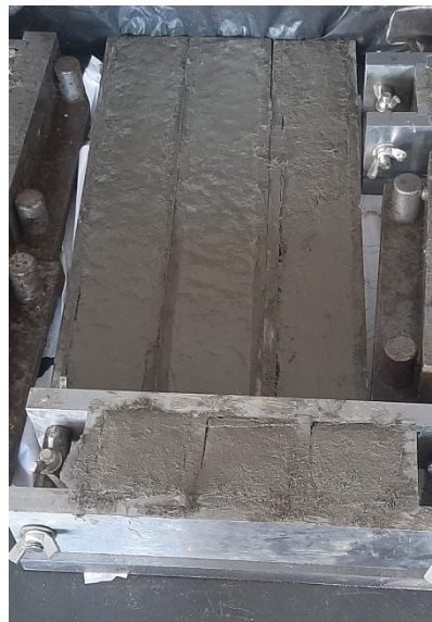
Figure 2. Poured fresh nanocalcite-doped ECC samples.
