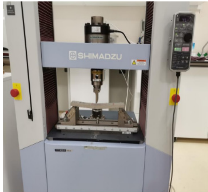
Figure 3. The flexural test set-up.
