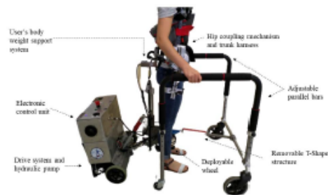
Fig. 1. General view of SWalker. The device consists of three major systems according to their functionality: (1) the drive system, (2) the user's weight support system, and (3) the user's safety support elements (such as parallel bars). The hip mechanism and trunk harness are elements of safety and stability for the patient as part of the weight support system. The T-shape frame and the deployable wheel are safety elements for the patient's transfer procedure. The electronic control unit consists of the control and communication systems. The hydraulic pump is part of the weight support system, but due to design requirements (weight and dimensions), it is housed in the traction structure.
