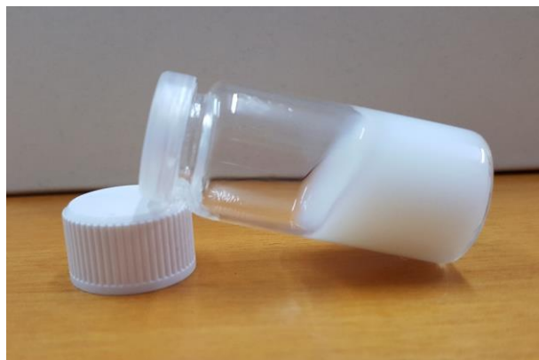
Figure 2.4. Appearance of the viscous 20 %w/w Soluplus dispersion in PBS pH 7.4 at 37 °C.
