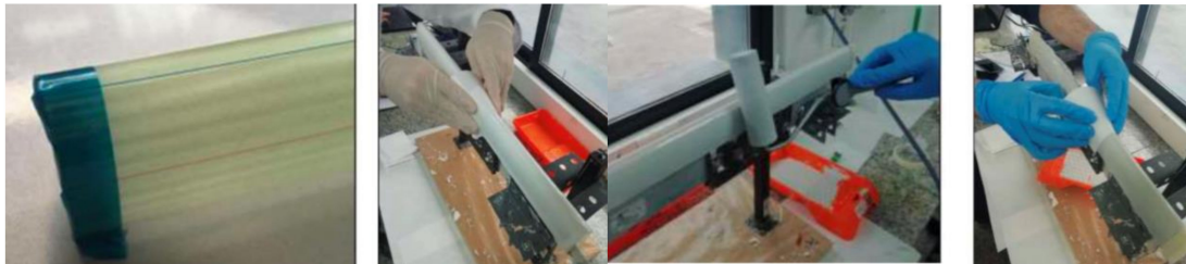
Figure 14. Application execution steps of RET testing coupons used in this work (DNVGL-RP-0171).
