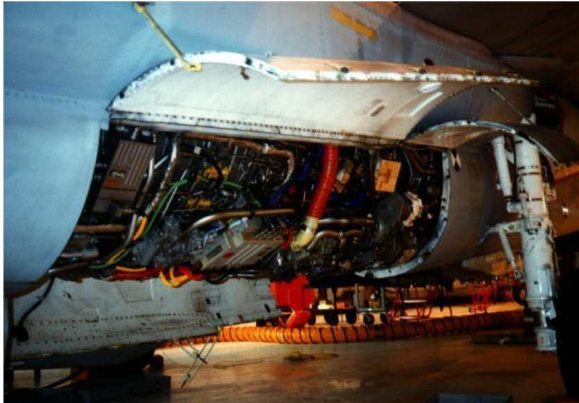
Figure 14. Engine nacelle of a typical fighter aircraft.
