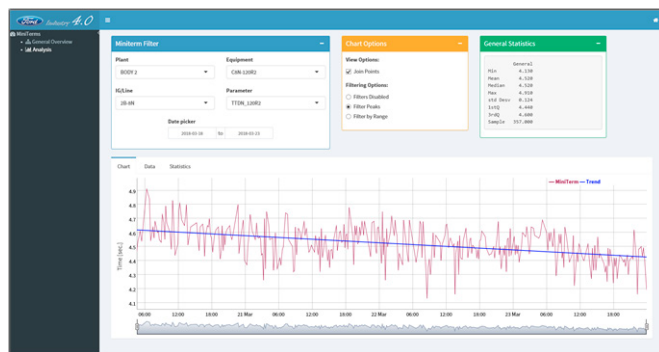
Fig. 5. Interface for Mini-term 4.0 . It analyzes mini-terms and sends e-mails to maintenance workers.
