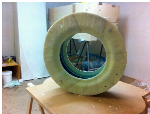
Figure 7. Glass fiber-reinforced epoxy (GFRE) mold developed for the manufacture of the membranophone shell.
