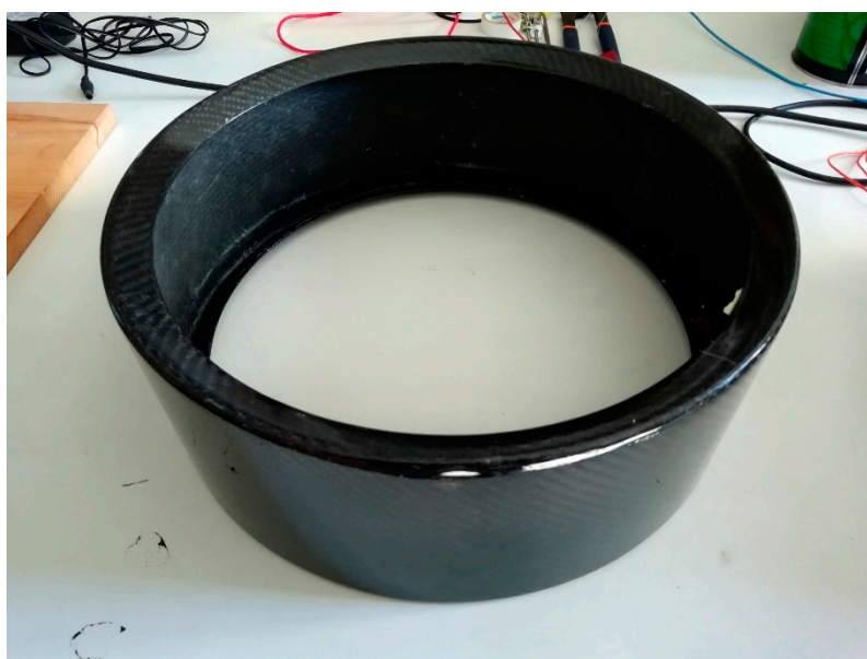
Figure 19. CFRE drum shell made for the experimental validation.
