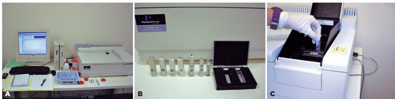
Figure 1. A) Spectrophotometer Perkin Elmer Lambda 35 UV/VIS used in this experiment. B) Different lens holders designed and built especially for placing the sample in the spectrophotometer. The three holders on the left are the holders for the pig lenses. C) Placement of lens holder with the crystalline lens directly in front and covering the complete entrance hole of the integrating sphere of the spectrophotometer.
