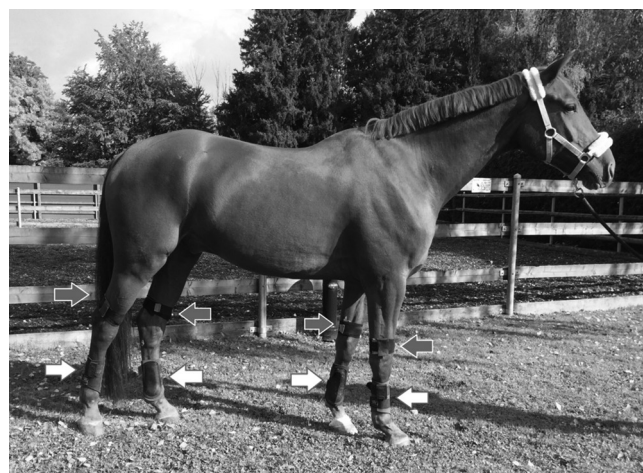
FIG 6: A horse instrumented with four standard brushing boots (white arrows), one on each third metacarpal/metatarsal bone and four custom-made elastic straps (grey arrows), two on the distal part of each radii just above the lateral radial epicondyle and two on the distal part of each tibia, in the groove just dorsal to the gastrocnemius tendon.
