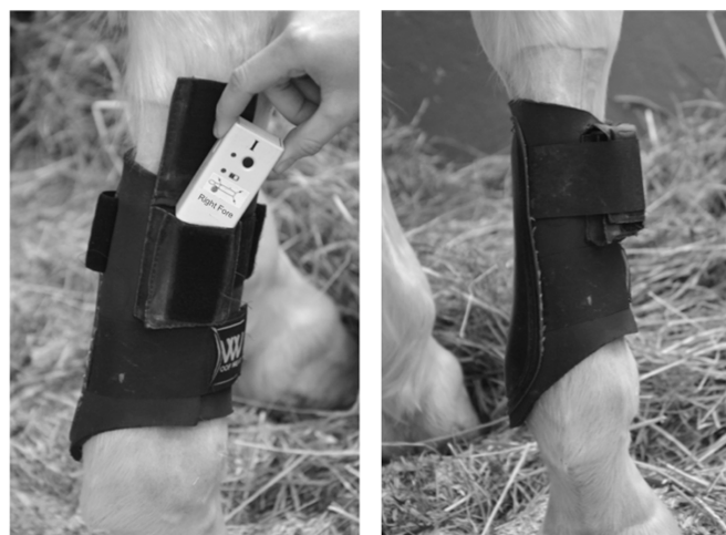
FIG 7: An exemplar of the custom fitted pouches, which are attached to the lateral aspect of each boot and strap to hold the IMU sensors firmly to reduce motion and to facilitate synchronicity with limb movement throughout the data collection period. Left: sensor is inserted into its pouch. Right: pouch is closed and Velcro strap is fastened over the sensor-pouch.
