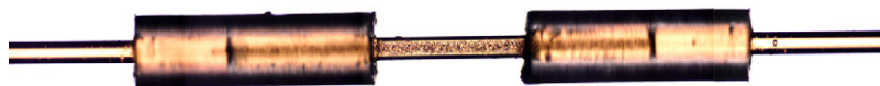
Fig. 1. Picture of the preconcentrator under 4× optic microscope. The preconcentration chamber houses the packed beads (30 μm average size in this case). The rest of the electrophoretic capillary, with noticeable lower internal diameter, extends towards both sides of the preconcentrator allowing the immobilization of the beads without the need of retaining frits in the system.
