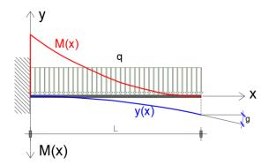
The maximum g rotation appears on the right end of the cantilever. Its value can be obtained with a definite integral between 0 and L of the function that results from dividing M(x) by the El constant.
