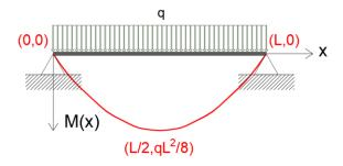
**b)** Obtain the explicit expression of M(x), using the provided coordinate system (y-axis oriented downwards).
