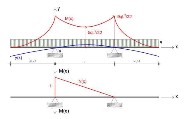
In this case, the **g** rotation on the left support can be obtained with a definite integral between 0 and L of the function that results from dividing the product of **M(x) N(x)** by the **EI** constant.
