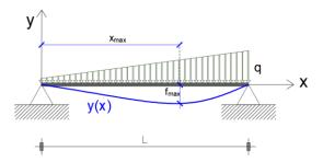
The load is not symmetrical. Thus neither M(x) nor y(x) are symmetrical. Hence, the maximum internal bending force and the maximum deflection will not appear in the middle of the beam. Answer the following:
