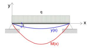
This rotation can be calculated dividing the area of the parabola M(x) (that was obtained in V01) by the constant value 2EI with a negative sign (counterclockwise rotation is considered positive by sign convention). Answer the following questions:
