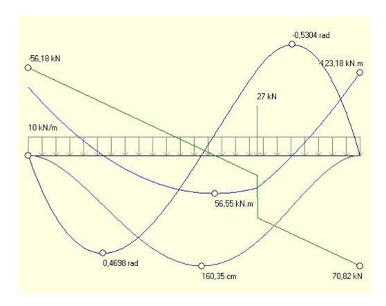
These functions are related to one another: The rotation function (represented with a dark blue curve is the derivative of the elastic deflection (purple). Similarly, the bending moment function (light blue) is the derivative of the rotation function; the shear-force function (green) is the derivative of the bending moment one, and the loading function (grey) is the derivative of the shear-force function.
