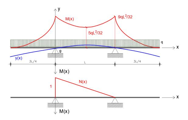
Find the value of the g rotation, using this time the Simpson's method to solve the definite integral:
