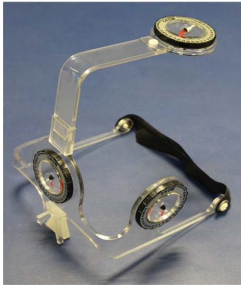
Figura 29. Goniómetro CROM ( Cervical Range of Motion Instrument ) (Performance Attainment Associates©, Lindstrom MN, USA) usado en el estudio.
