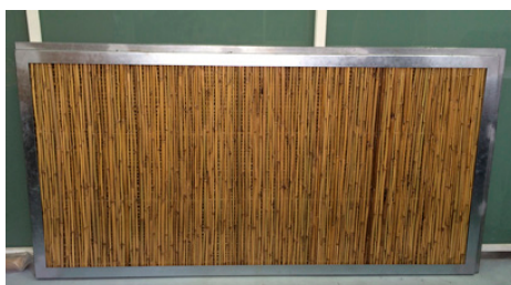
Figure 3. Bamboo floor panel 5
