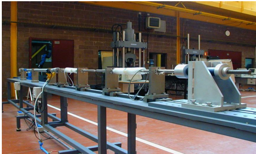
Figure 6. Split Hopkinson Tension Bar apparatus as installed in the Universidad Carlos III de Madrid Engineering Laboratory.
