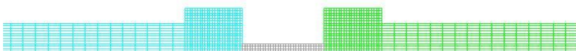
Figure 18. Structured mesh in the modified SHTB model when the cross-sectional area of the bar ends which are in contact with the specimen is increased (Model-2).
