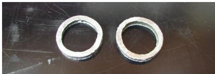
Figure 13. 30-mm inner diameter and 3-mm thick damping disks
