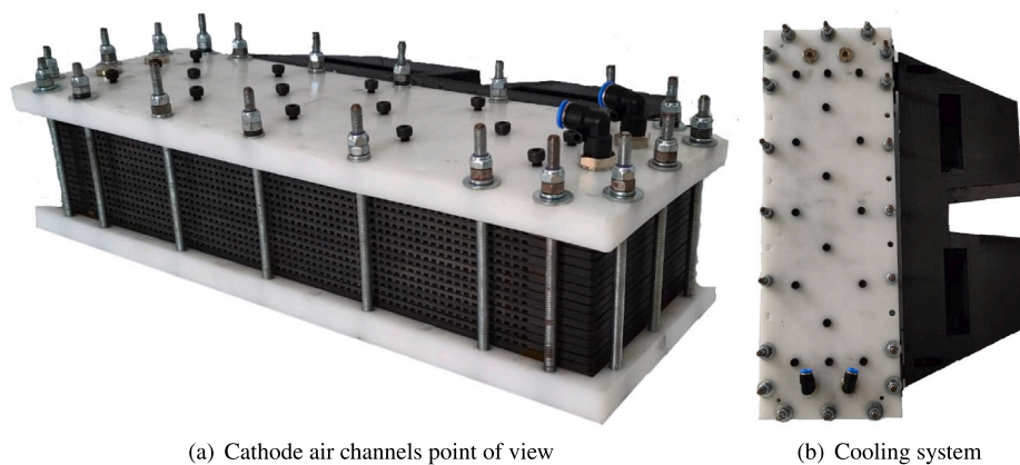
Fig. 4. Assembled stack with the air cooling system installed.
