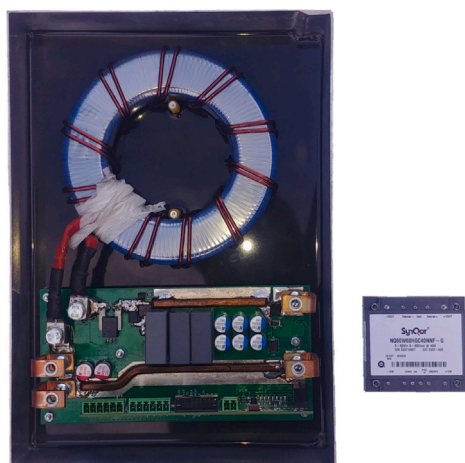
Fig. 6. Comparative of both DC converters used, ad-hoc DC-DC converter (left) and commercial converter (right), both for up to 1 kW.
