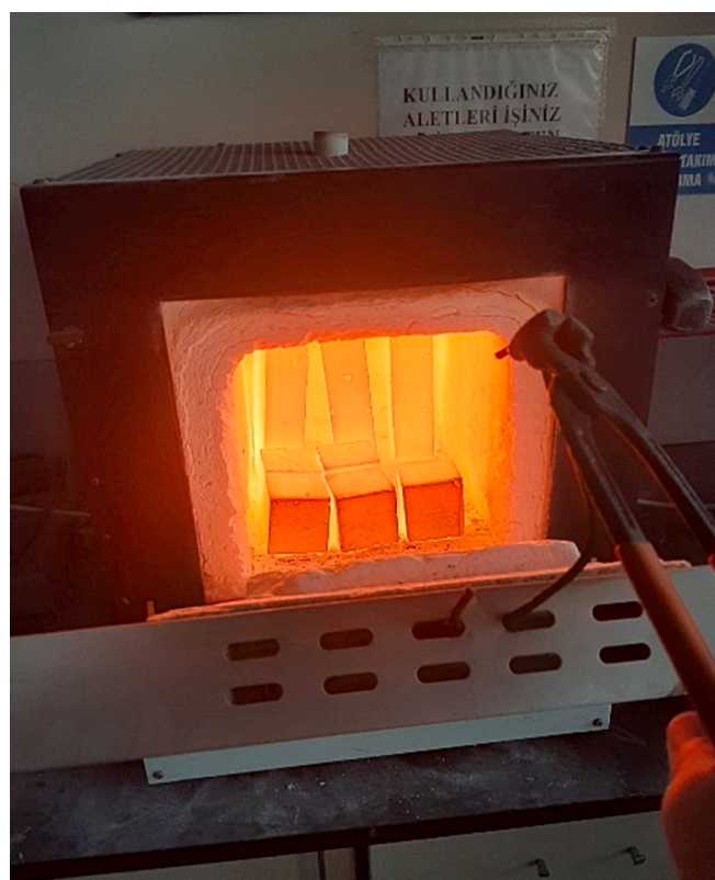
Fig. 3. Cube and prism geopolymer mortar samples placed in a high-temperature furnace.
