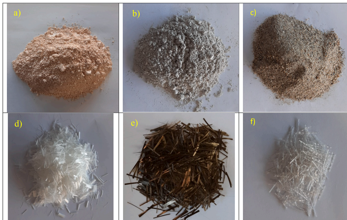
Fig. 1. Images of materials and fibers used in geopolymer mortar blends: (a) Metakaolin, (b) slag, (c) sand, (d) PVA, (e) BS, and (f) MSP.
