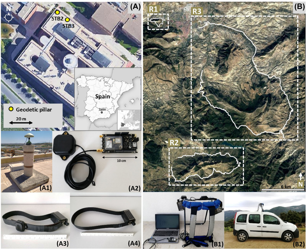
FIGURE 2 A) Location of geodetic pillars STB2 and STB3 for the static test carried out at the Campus of the University of Jaén, Spain, from 16–25 February 2021 showing the geodetic global navigation satellite system (GNSS) receiver and antenna (A1), the low-cost GNSS receiver and active patch antenna (LCR; A2), the multi-frequency GNSS collar (MFC; A3) and the single-frequency GNSS collar (SFC; A4). B) Routes R1, R2, and R3 for the kinematic test carried out in Jaén, Spain, in June 2021 and 2022 showing the equipment for route R1 (LCR, MFC and SFC, laptop and backpack; B1) and equipment and vehicle for routes R2 and R3 (B2).
