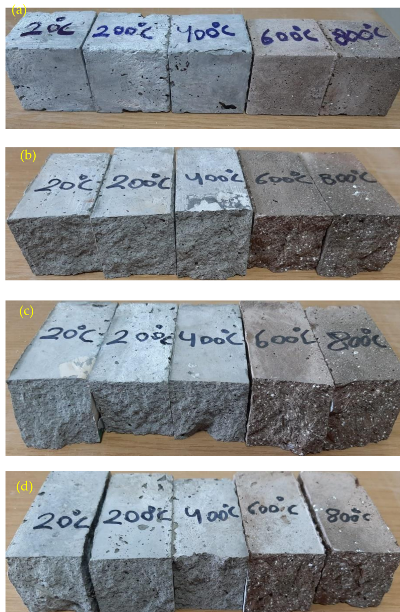
Figure 15. Fly ash-based geopolymer samples exposed to various temperature effect (a) 0 BF; (b) 4 BF; (c) 8 BF and (d) 12 BF.
