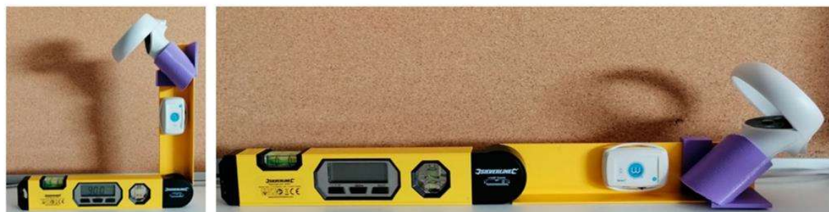
Fig. 3 A controller holder was 3D printed, which allowed the controller to be reliably rotated by 90°. The controller could then perform three orthogonal rotations about a single axis. Both Oculus Touch v2 and the inertial sensor were attached to the digital goniometer
