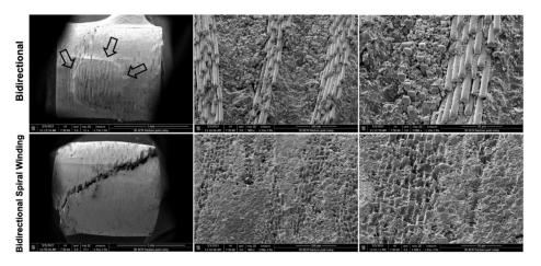
**Figure 2.** Representative scanning electron microscopy photos of bFRC and bswFRC fractures at different magnifications (×31, ×500 and ×1000). Black arrows indicate a shear fracture in bFRC sample.
