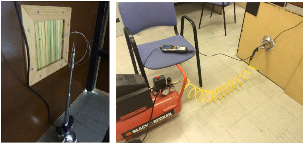
Fig. 11. Thermal anemometer and mounting system for the air permeability test.
