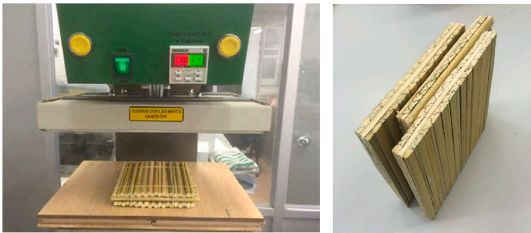
Fig. 5. Process of pressing the whole reeds.
