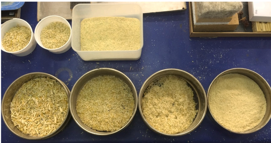
Fig. 2. Sizes and sieves of shredded fibers.
