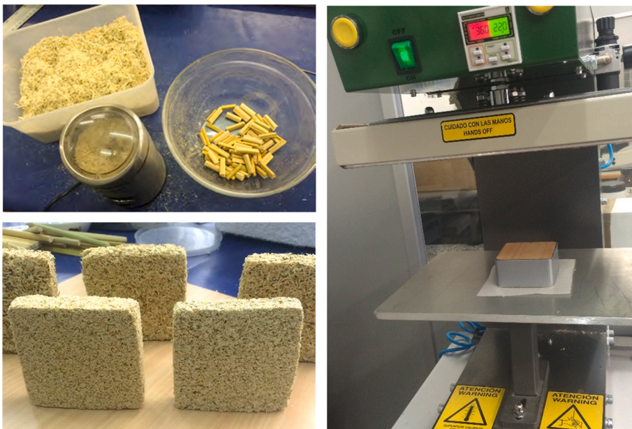
Fig. 3. Process of crushing and compacting the fibers.
