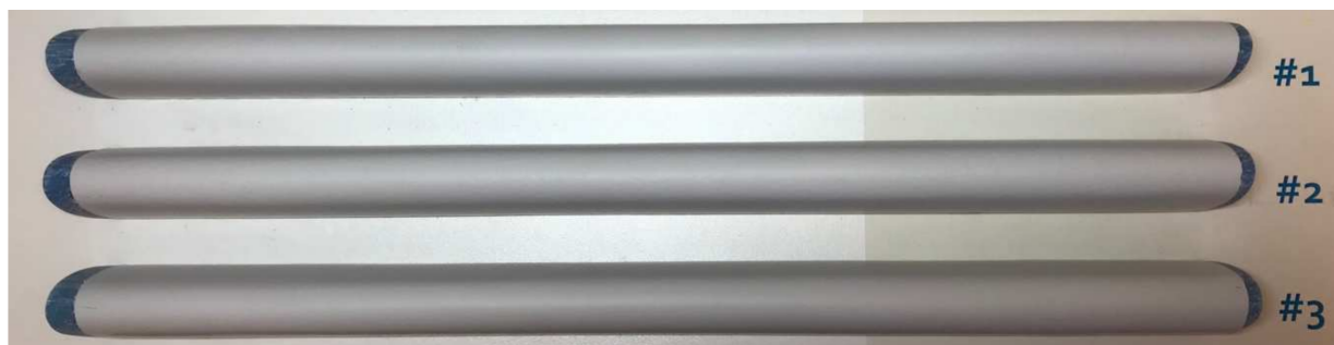
Figure 6. The three rain erosion samples at the start of the test. The high-speed tip end is on the right-hand side of the figure.
