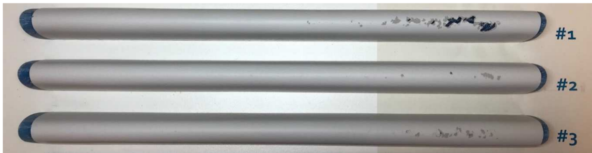
Figure 9. The test samples after 11 h in the rain erosion test rig at a rotational velocity of 1000 rpm.
