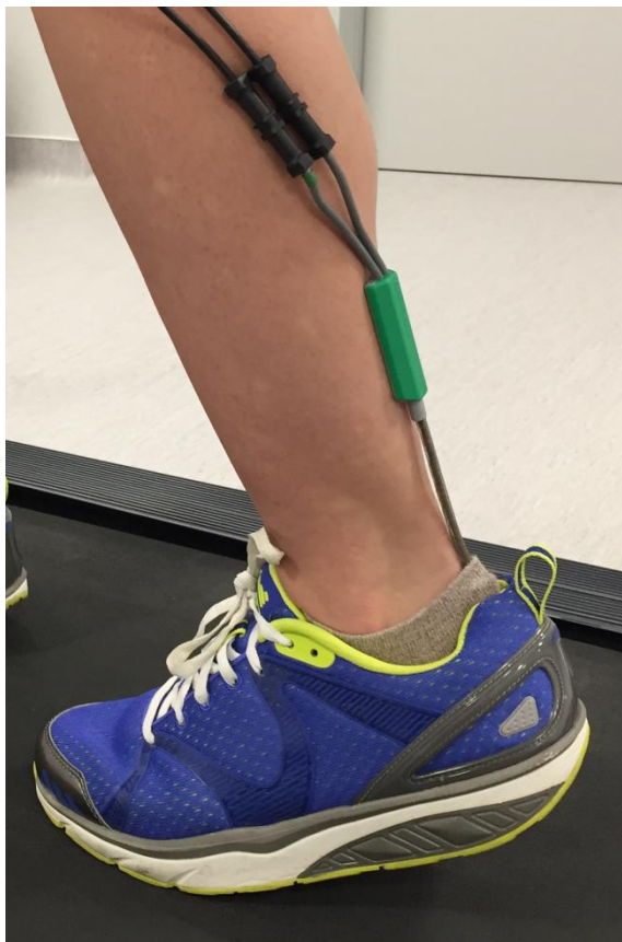
Figure 1. Unstable test shoe used in the study (MBT, model AFIYA 5). The illustration shows the electronic goniometer array used for assessing the ankle range of movement.
