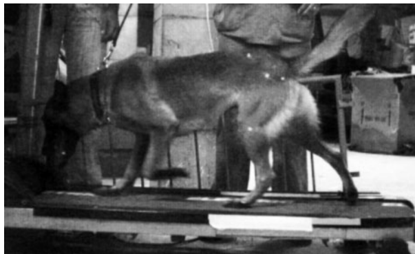
Figure 1. Frame obtained from the high-speed video camera. Note the retroreflective markers positioned over anatomic references.
